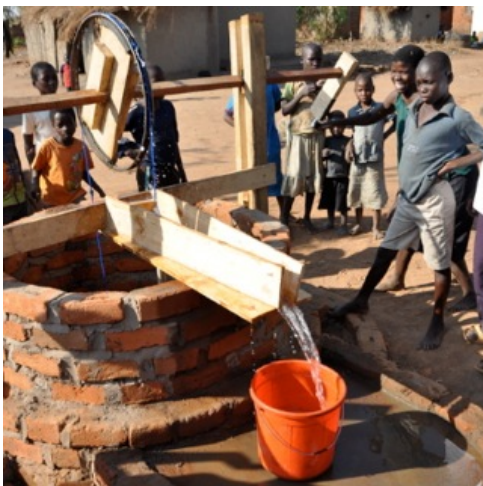
Figure 9: Photograph of the Abakus Pump Without Protection
